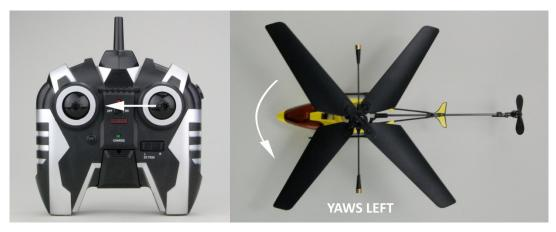
Moving the stick to the right will turn (yaw) the nose of the helicopter to the right about the axis of the main shaft. This is accomplished by increasing the speed of the lower main rotor blades while decreasing the speed of the upper main rotor blades.
