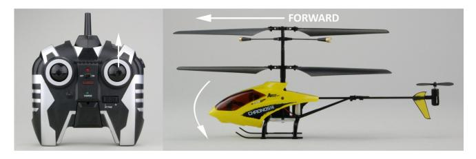
Pulling the stick backward will run the tail motor in the opposite direction so it pitches the tail of the helicopter downward, allowing the helicopter to be flown backward.
