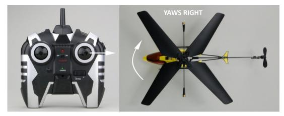
The rudder (steering) trim is used to help keep the nose of the helicopter from constantly rotating to the left or right when in hover and with no right-hand stick input. For example, if the nose of the helicopter rotates to the right when in hover, add left rudder trim by pressing the left-hand rudder trim button until the nose of the helicopter stays as close to straight as possible with no input from you.
