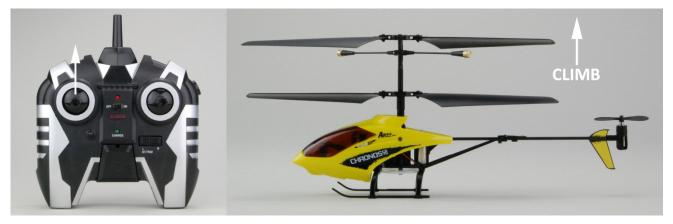
Decreasing the speed of the main rotor blades by lowering the left-hand stick will cause the model to descend.
