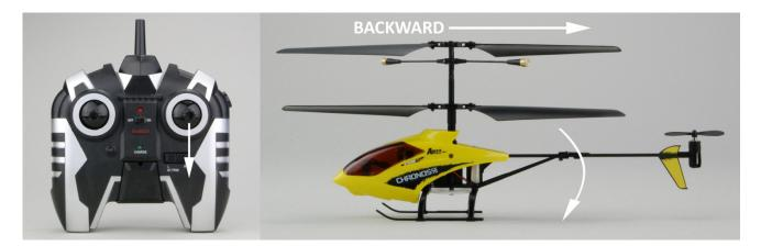
Moving the right-hand stick to the left will turn (yaw) the nose of the helicopter to the left about the axis of the main shaft. This is accomplished by increasing the speed of the upper main rotor blades while decreasing the speed of the lower main rotor blades.
