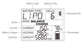
Battery Type: select the chemistry of the battery to be processed.
