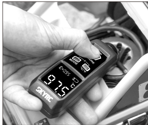
Measure the engine temperature
