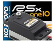
The RSx one10 Type-S is a "low-profile" Servo from KoPropo with the target to have a high performance for a lower price. The Servo can be used with 6V and also with 7,4V from a LiPo and includes metal gears, a heat sink middle case, core-less motor and dual bearings.
