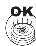
Good Plug Element glows when tested.
