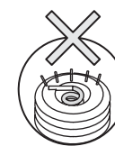
Bad Plug Element may be damaged or broken if it doesn't light up completely.
