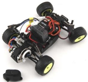
Below the stock motor is on the right. Using the backside of the side cutters carefully push the pinion away from the motor. The pinion is made of plastic and will come off without much trouble.
