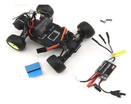
Different view with the ESC mounted on the servo tape.
