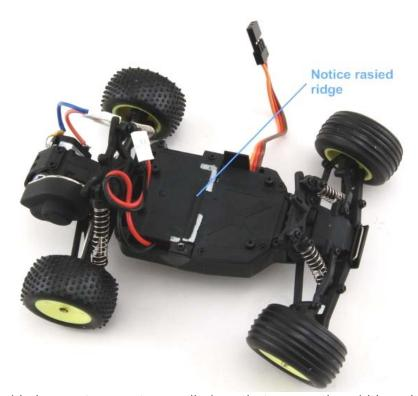
Using double sided servo tape, cut a small piece that covers the width and long side of the receiver. Locate the servo tape just to the rear of the ridge. We put the two silver L shapes for reference, on the chassis to highlight and show you the location for the receiver.
