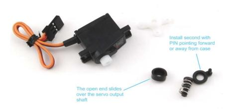
Servo with saver installed should look like the figure below.
