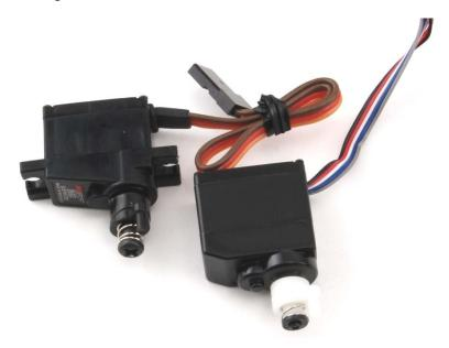
Using the side cutters, we need to carefully remove the normal servo mounting ears.
