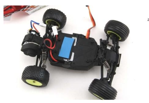
The receiver has been installed.
