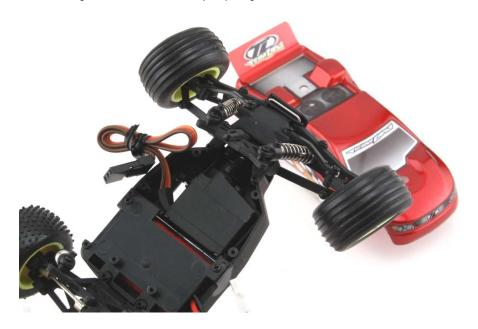
Reinstall the servo cover now. Using the four (4) screws removed in step #4.
