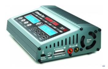
SKYRC Ultimate Duo is a twin-channel charger with two independent circuits which can charge two different kinds of batteries simultaneously. The Ultimate Duo 700W features the so-called AUTO function that set the feeding current during the process of charging or discharging.
