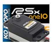
The RSx one10 Type-S is a "low-profile" Servo from KoPropo with the target to have a high performance for a lower price. The Servo can be used with 6V and also with 7,4V from a LiPo and includes metal gears, a heat sink middle case, core-less motor and dual bearings.
