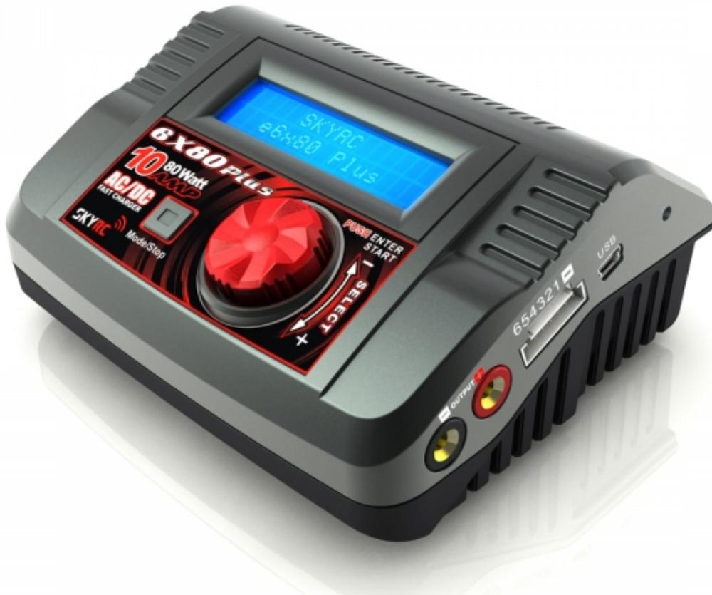
SkyRC 6x80 Plus is a high-performance, micro processor control charge/discharge station with battery management suitable for use with all current battery types. With integral equalizer for six-cell, Lithium- Polymer (LiPo), Lithium-Ferrum (LiFe) and Lithium-Ion (LiIon) batteries. Maximum 10A charge current; maximum 80W charge power; can be powered by a 12 Volt car battery or from 100V-240V via the built in switch-mode power supply.
