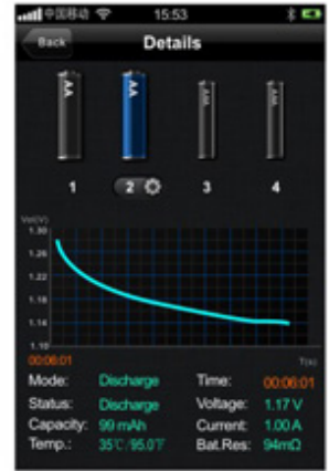
Discharge voltage curve, battery internal resistance & other information
