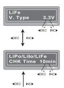
To change the default values, press the Start/ Enter key once. The value to be adjusted will blink indicating it can be edited. Use the Inc/Dec keys to adjust the value to the desired setting, then press the Start/Enter key once to save your changes for that value
