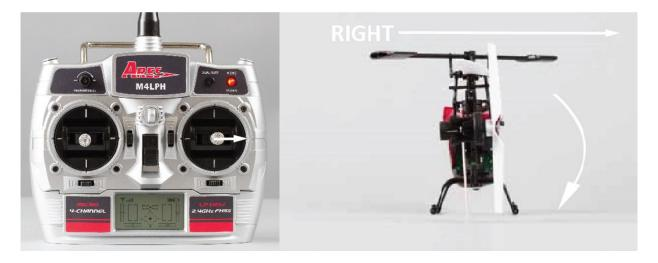
The aileron trim lever (located immediately below the right-hand stick) can be used to help keep the helicopter from drifting left or right when hovering and with no right-hand stick/aileron control input. For example, if the helicopter drifts to the right when hovering add left aileron trim by pressing the lever to the left until the helicopter hovers as level as possible without drifting to the right.
