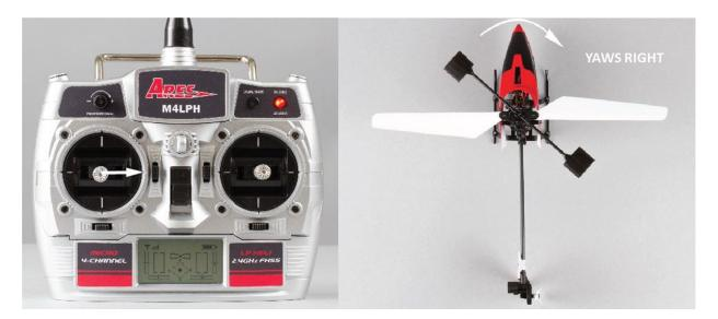
The rudder trim lever (located immediately below the left-hand stick) can be used to help keep the nose of the helicopter from turning (yawing) to the left or right when 'hovering' and without any left-hand stick/rudder control input. For example, if the nose of the helicopter turns to the right when hovering add left rudder trim by pressing the lever to the left until the nose of the helicopter stays as close to 'straight' as possible with no further rudder control/trim input.
