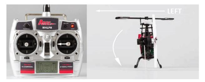
Moving the right-hand stick to the right will roll the helicopter to the right, allowing it to be flown to the right. This is accomplished by having the aileron (left-hand) servo push the swashplate upward.
