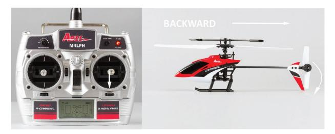
The elevator trim lever (located immediately to the left of the right-hand stick) can be used to help keep the helicopter from drifting forward or backward when hovering and with no right-hand stick/elevator control input. For example, if the helicopter drifts forward when hovering add back/up elevator trim by pressing the lever downward until the helicopter hovers as level as possible without drifting forward.
