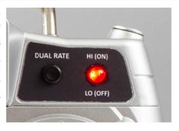
When the LED indicator is OFF the control rate is set to 'LO' and the maximum control rates/values will be reduced for the aileron and elevator channels. This is typically preferred by (and recommended best for) low-time and other pilots interested in a reduced amount of control authority that allows for even smoother and more easily controlled hovering/flying.
