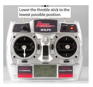
Moving the left-hand stick to the left will turn (yaw) the nose of the helicopter to the left about the axis of the main shaft. This is accomplished by decreasing the speed/RPMs of the tail rotor.
