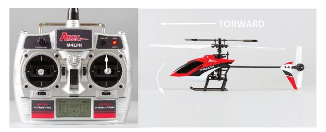
Pulling the right-hand stick backward will pitch the tail of the helicopter downward, allowing it to be flown backward. This is accomplished by having the elevator (right-hand) servo push the swashplate upward.
