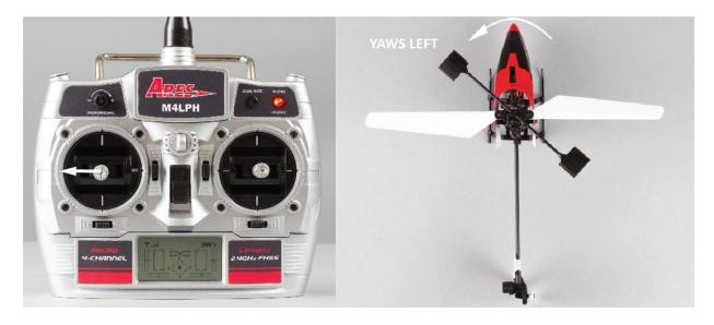
Moving the left-hand stick to the right will turn (yaw) the nose of the helicopter to the right about the axis of the main shaft. This is accomplished by increasing the speed/RPMs of the tail rotor.
