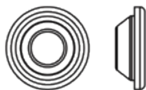
AX30112 Shock Diaphragm 13x4.5mm x4
