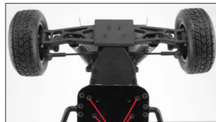
Servo Removal Remove these 4 screws
