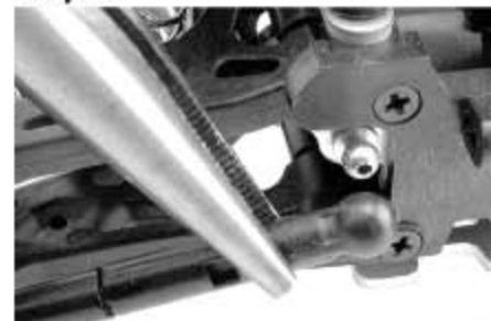
Using pliers, remove tie rod end as pictured.
