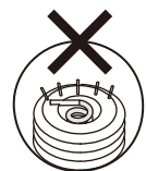
X Bad Plug Element may be damaged or broken if it doesn't light up completely.
