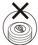
X Bad Plug Element is broken or doesn't light up at all.
