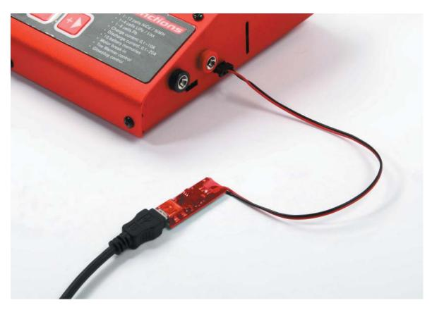
First connect the USB interface with the delivered USB cable to a free USB port on your PC. You will be promted to install the driver for the interface. Please use the driver delivered on the USB stick. If the driver is installed correctly the red LED on the interface will light up. You can also install LogView now. Instructions for using LogView the first time you find in your OVERLOADER2 instruction manual.
